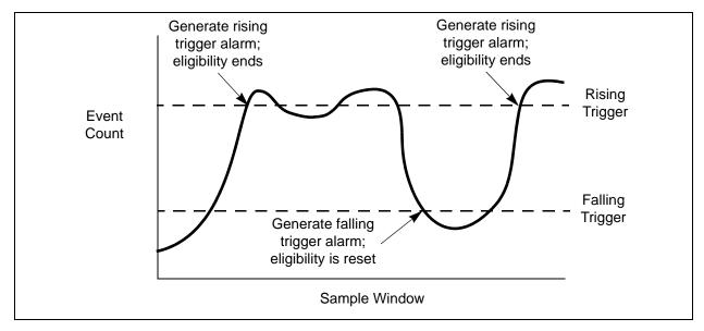
Figure 4-8. Port Threshold Alarm Example
